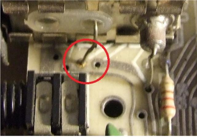
Step 3. Connect a new wire. Solder a short piece of wire to the modulator output pin, then feed wire through plastic insulator on side of modulator and finally connect wire to the pad where you disconnected the modulator input in step 1.
