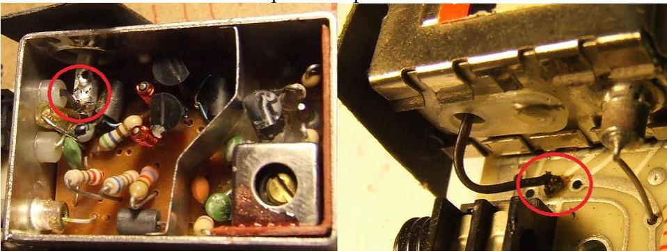
Method 2. connect a flying lead, instead of modifying the modulator a suitable lead can be connected directly to the ZX81, disconnect the modulator input wire, you should connect the GND (screen/shield) of your lead to a suitable gnd on the ZX81, probably the easiest point is the modulator casing itself. Then you should connect the video (signal) of your lead to the pad where you disconnected the modulator input from.
