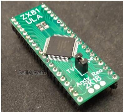
The replacement ZX81 ULA module is designed with modern surface mount components and recreates the logic of the original Ferranti Chip.
